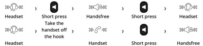
You are in conversation with the headset and the handset is not hang-up, you can switch between following audio modes by short pressing on the loudspeaker/hands-free key:
